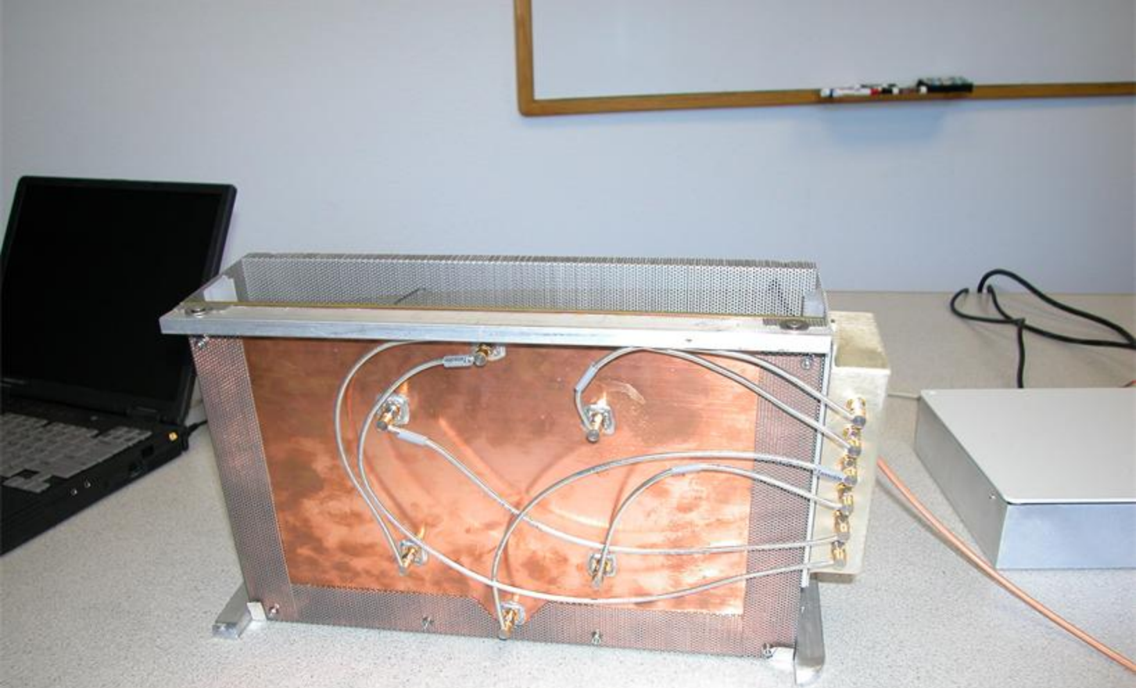
Six Antenna PCB Array Module with Switch Attached Bottom View
