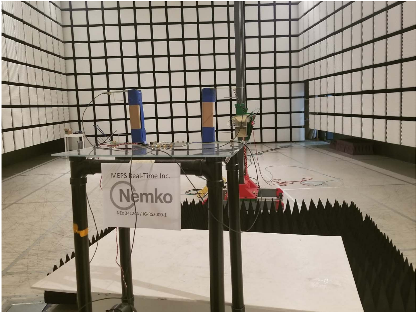
Figure 1.1-3: Radiated Emissions setup photo Back (1GHz-18GHZ)
