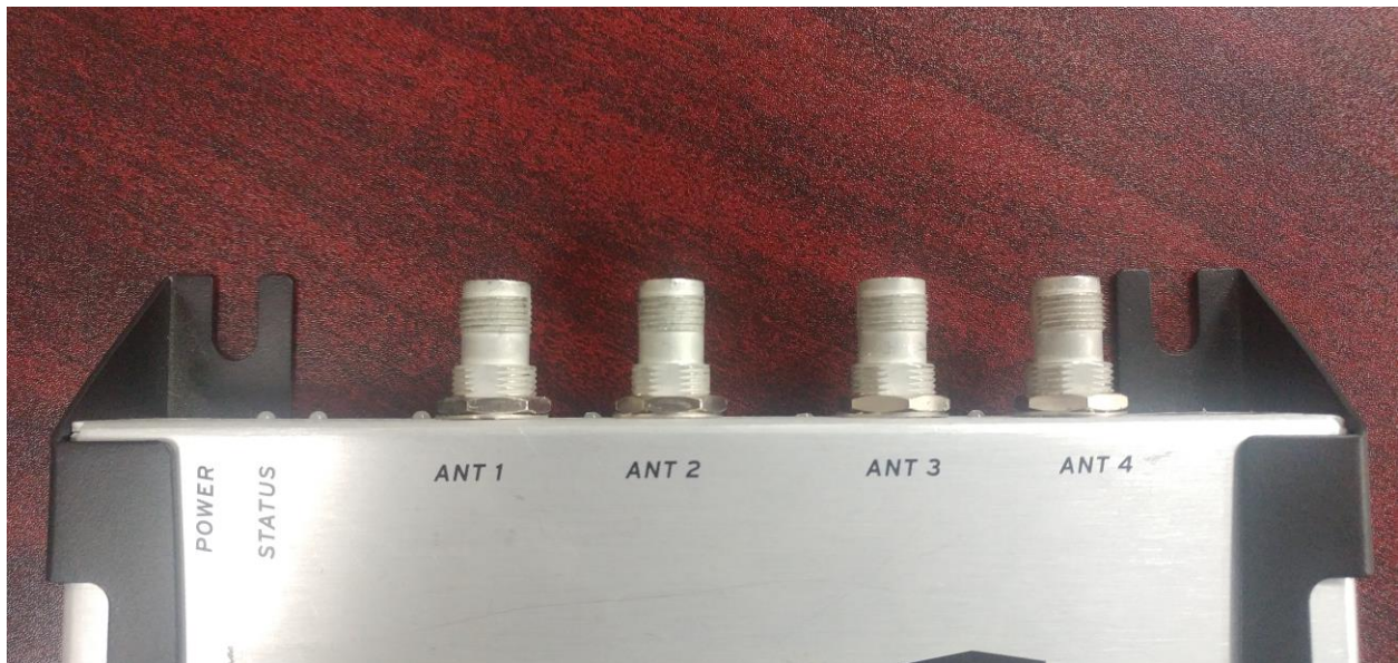
Figure 3. IG-REV-1 Antenna Ports, Power and Status Indicators
