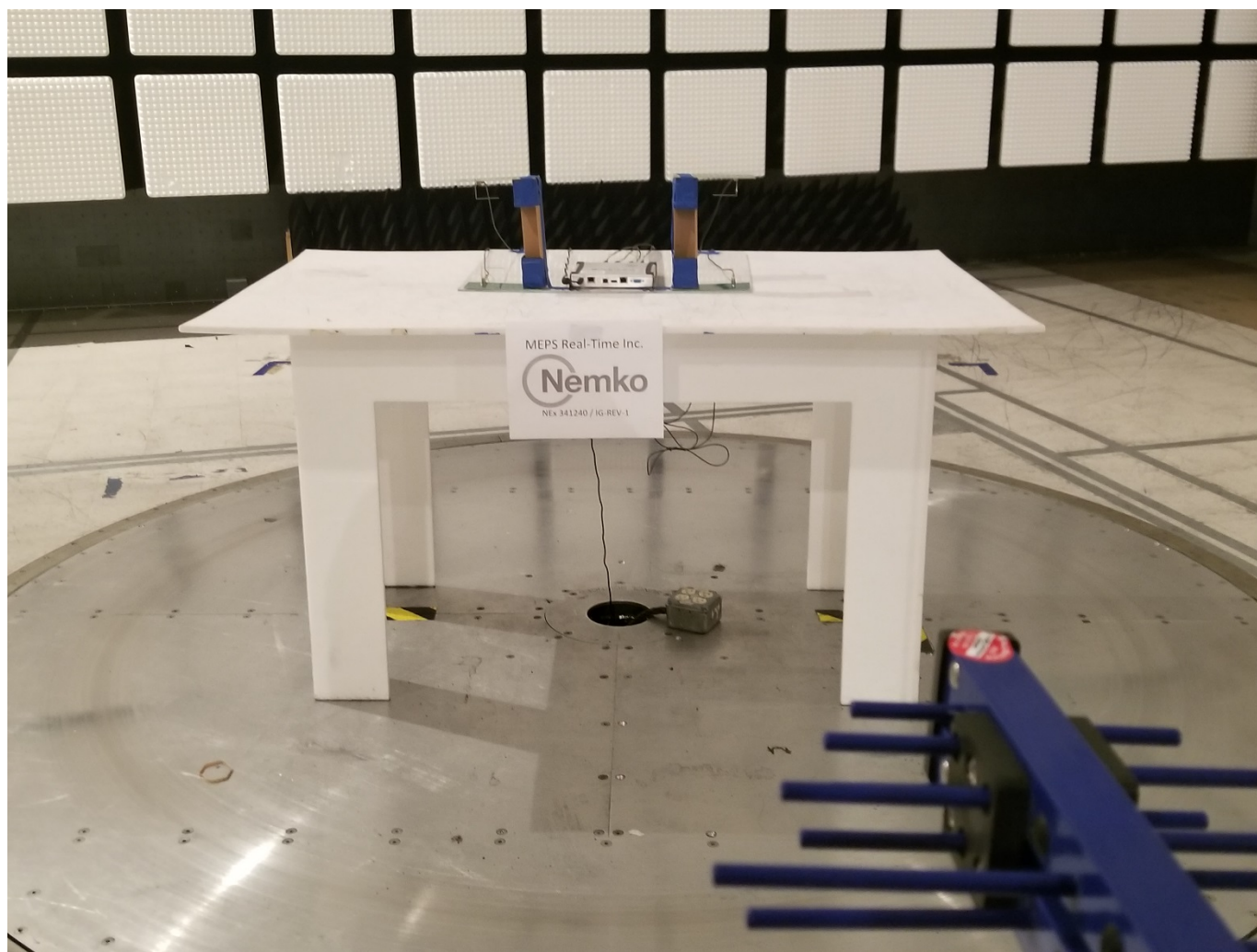
Figure 1.1-2: Radiated Emissions setup photo Front (30MHz-1GHZ)
