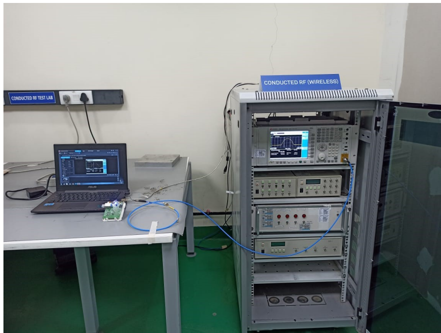
Figure 8 Photograph of Conducted RF measurements test setup - Antenna port
