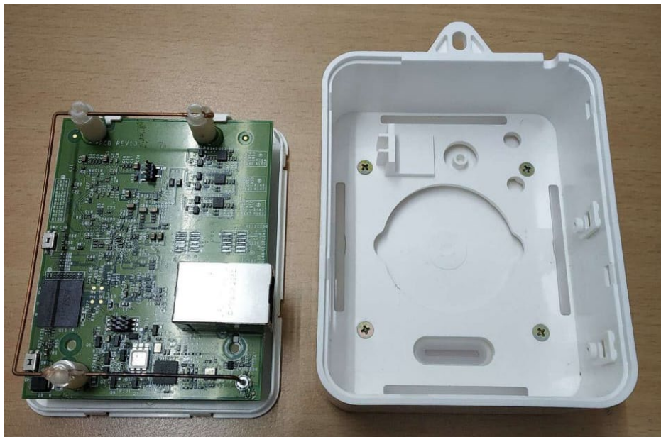
Figure 5 Photograph of Pella Insynctive Bridge- Internal – Along with enclosure
