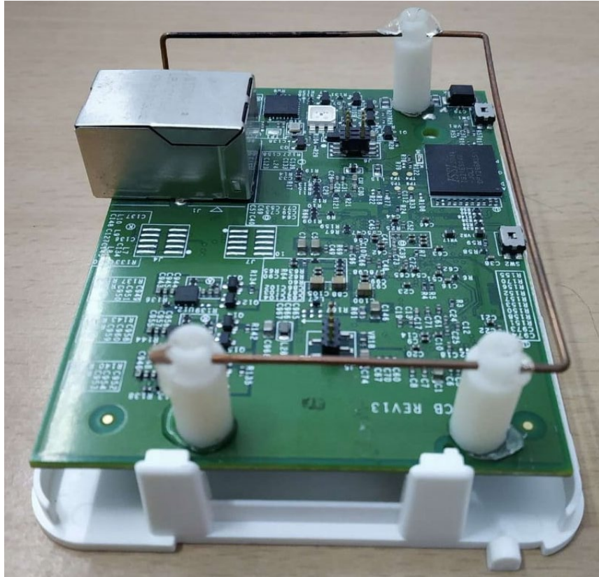
Figure 18 Photograph of Monopole Copper-Clad antenna installed in the product
