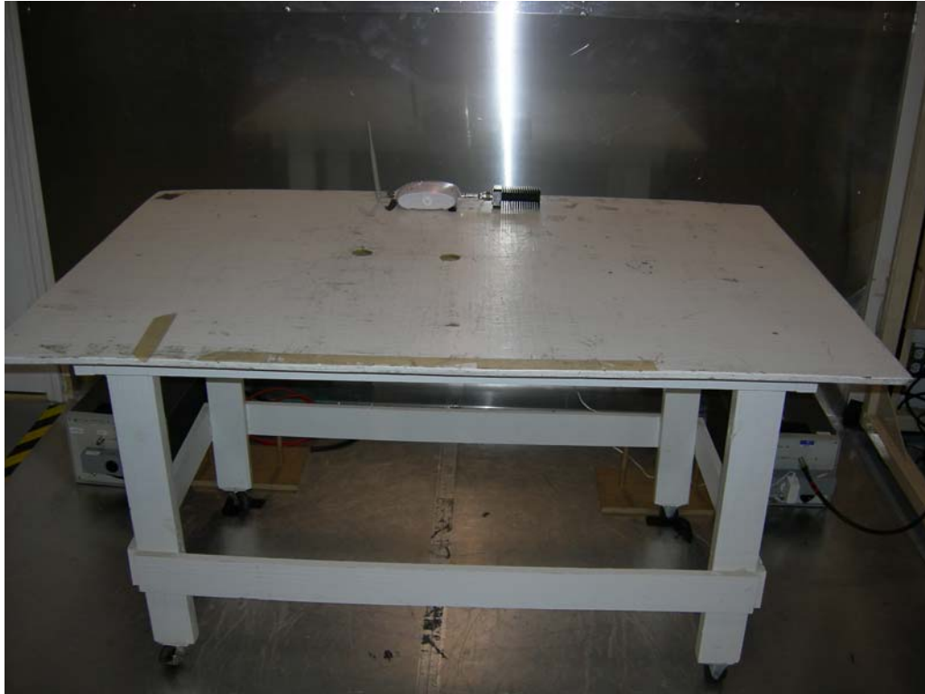
Figure 6: Test Setup – AC Power line Conducted Emissions
