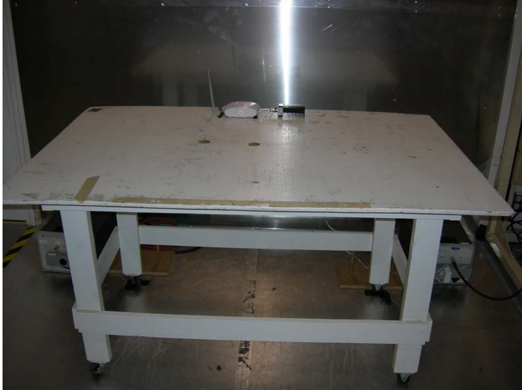
Figure 6: Test Setup – AC Power line Conducted Emissions
