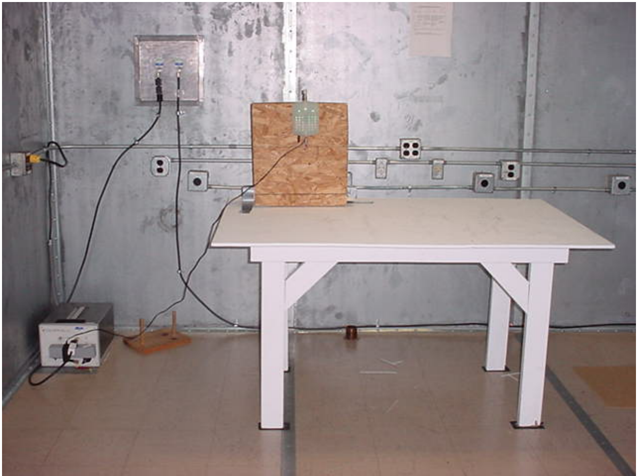
Figure 3: Conducted Emissions – Front View
