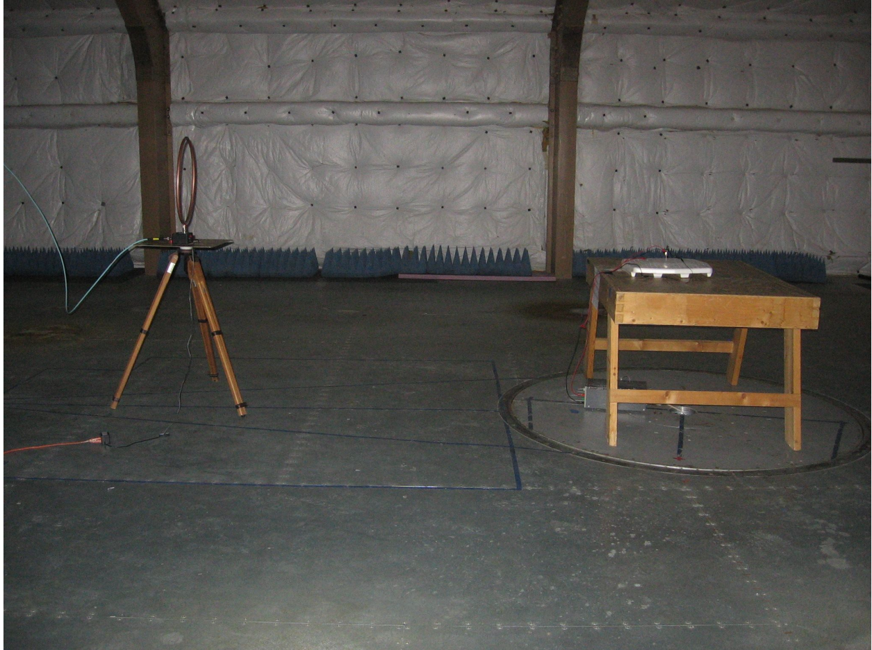
EUT set up in OATS, 9kHz – 30MHz Powered with external DC supply
