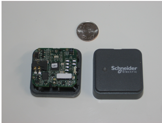
EUT PCB in case (top)
