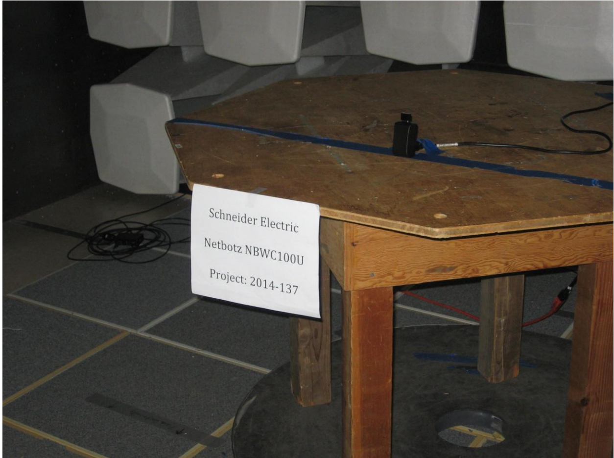
EUT set up in chamber, 30-1000MHz scans
