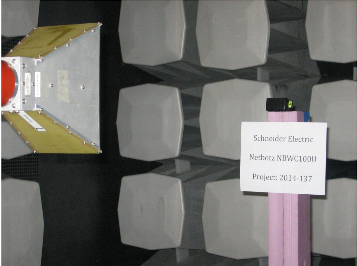
EUT set up in chamber, Above 1000MHz scans
