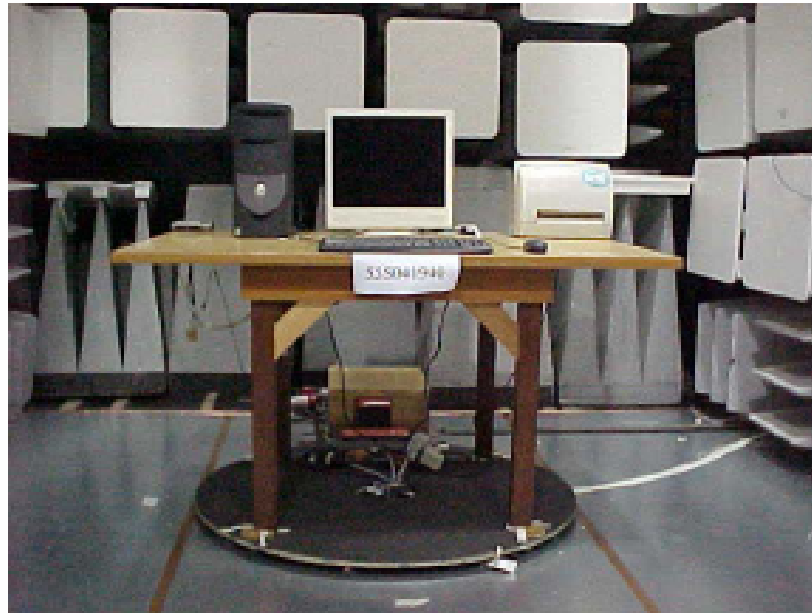
Radiated Emission Setup (front view)
