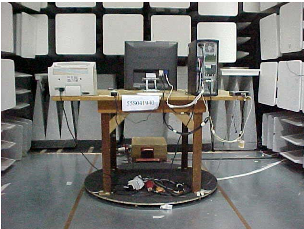
Radiated Emission Setup (rear view)
