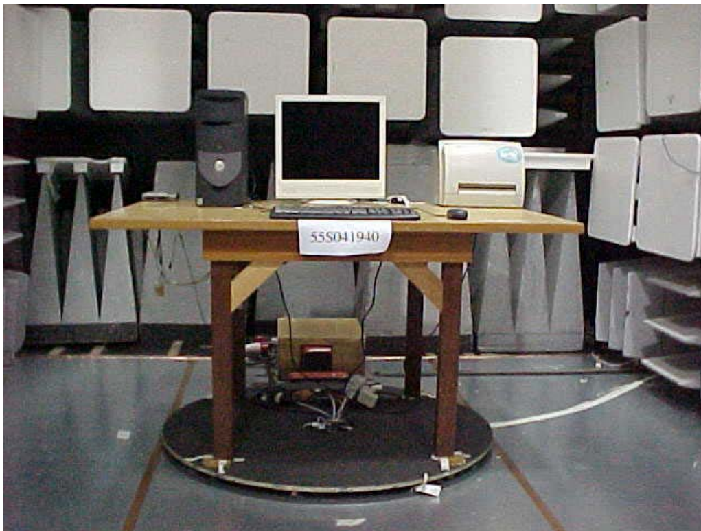
Radiated Emission Setup (front view)
