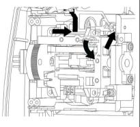
Assemble the centering cam into the throttle gimbal of mode 1 transmitter and set the spring in the center control part and the centering cam with tweezers
