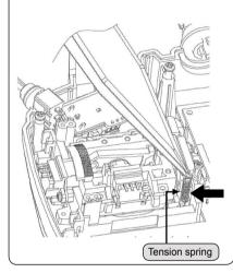
Screw the disassembled tension control bolt from the elevator gimbal of mode 1 transmitter into the throttle gimbal and adjust the bolt for the desired control
