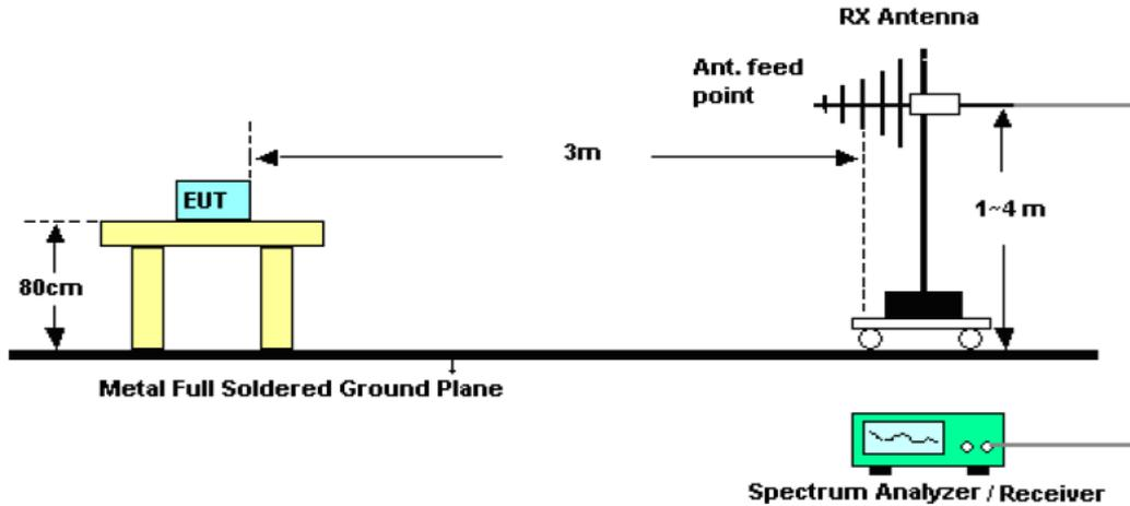
For radiated emission from above 1GHz
