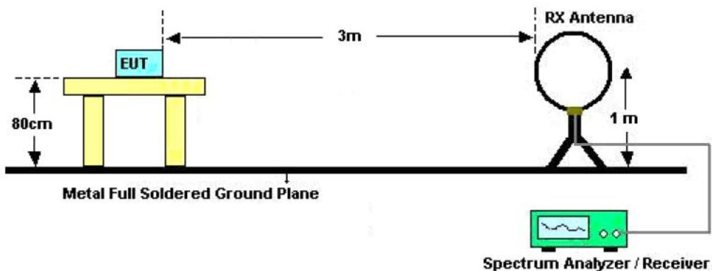
For radiated emission from 30MHz to 1GHz
