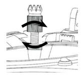
Both sticks can be adjusted in length: By holding the lower half and turning the upper part of the knurled handle, the screw is loosened. The control stick is extended or shortened by turning it up or down
