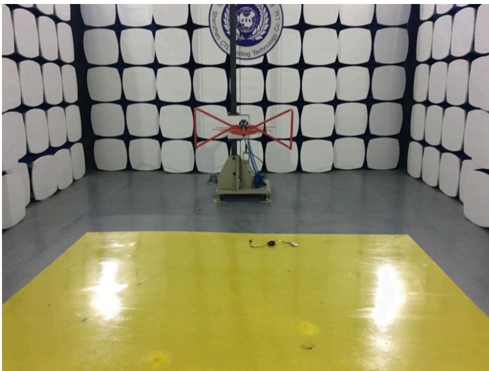
Radiated emission 30M~1G
