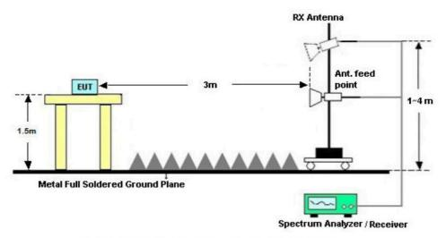
Conducted Measurement Setup NGCAL TESTING
