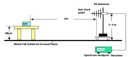
For radiated emission from above1GHz
