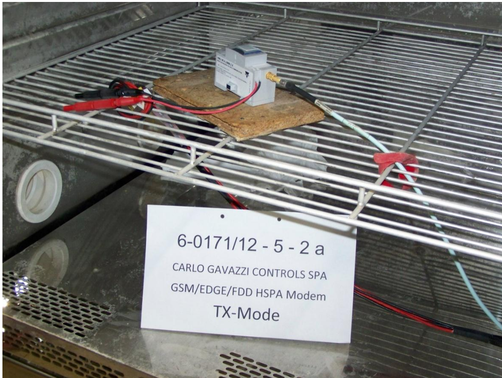
Conducted RF-measurements at the Radio laboratory 1 (in the climatic chamber), test setup 5
