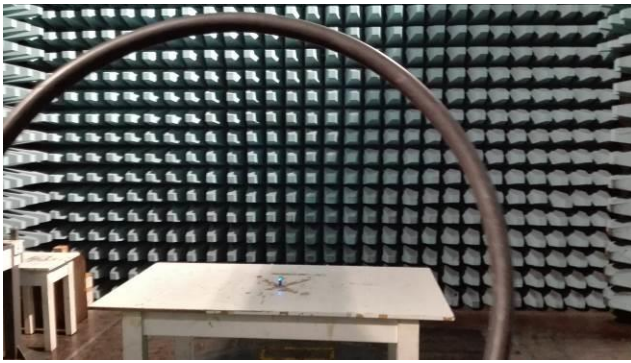
PHOTO N°3 SETUP FOR RADIATED MEASUREMENT <1GHz
