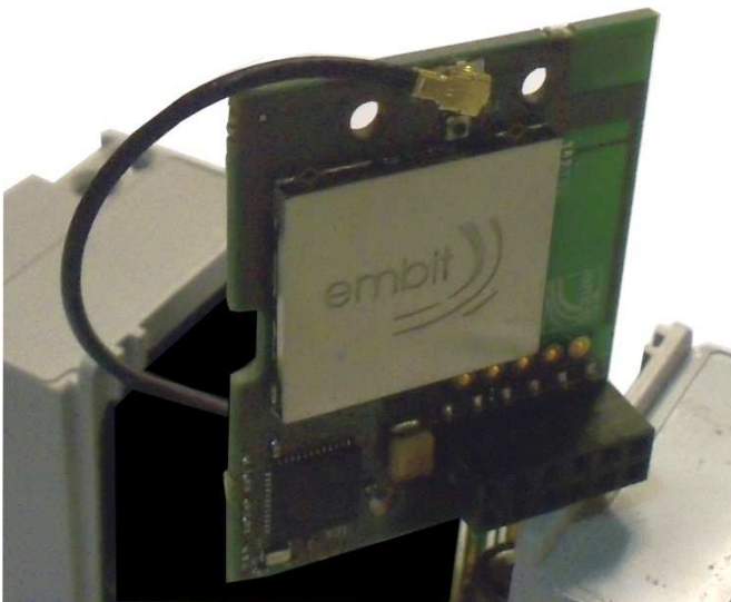
View of internal connector on radio board, for external antenna
