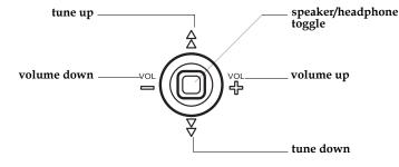
Press and hold the tuning buttons to scan up or down the frequency range and stop when a station is found.
