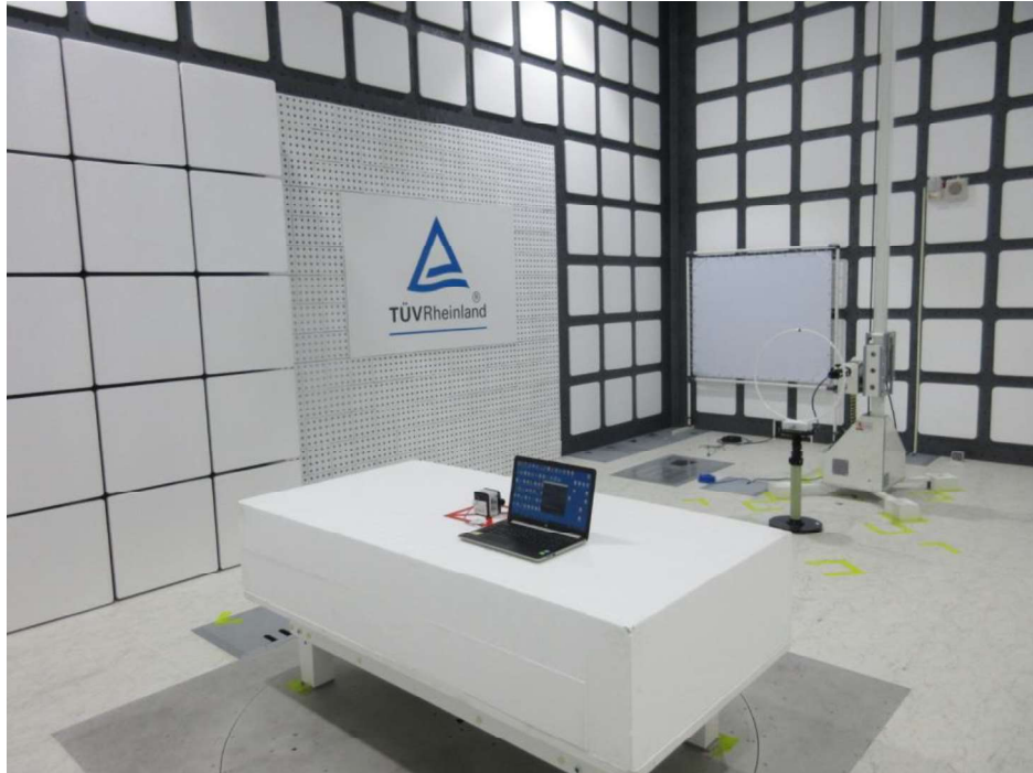
Photograph 5: Set-up for Spurious Emissions (Back View 3)
