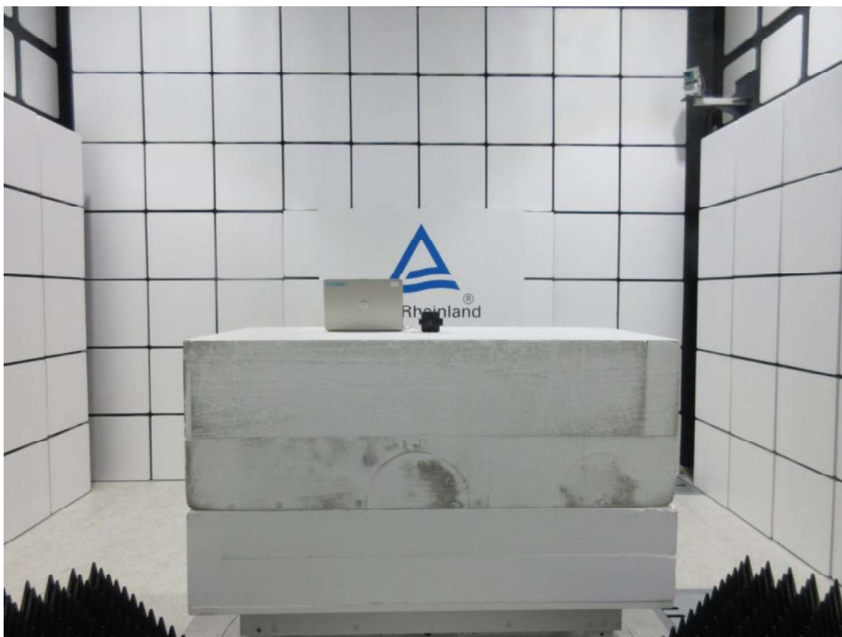
Photograph 2: Set-up for Spurious Emissions (Front View 2)
