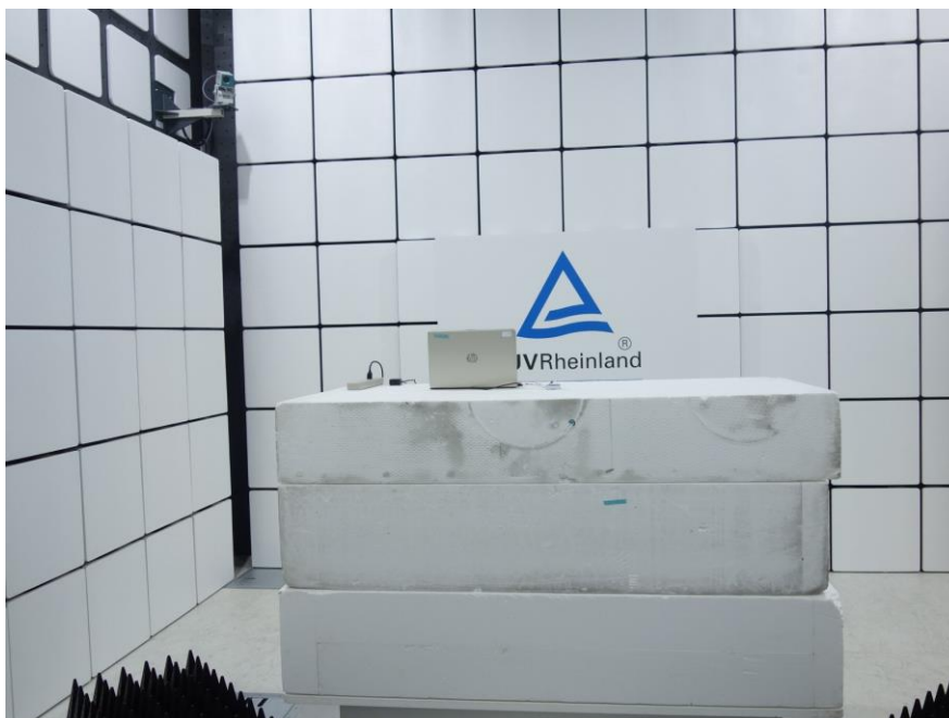
Photograph 2: Set-up for Spurious Emissions (Front View 2)
