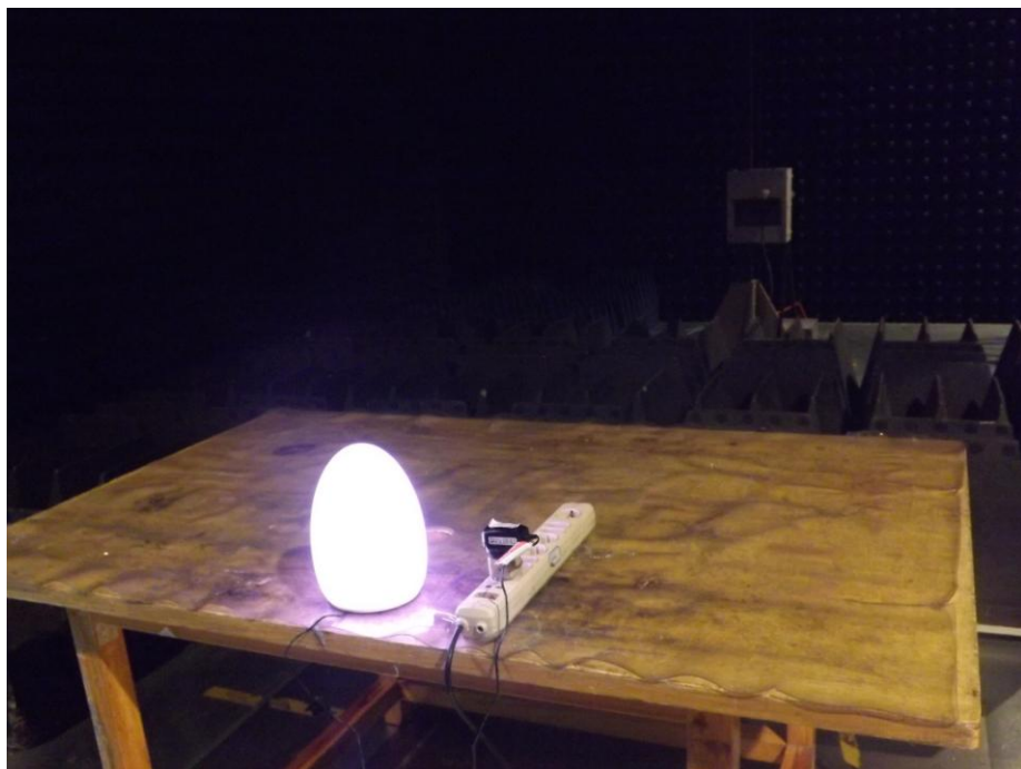
Test frequency above 1GHz at test site 1#
