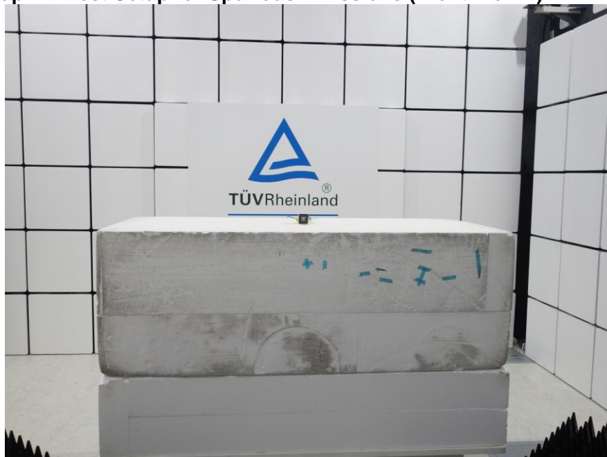
Photograph 2: Test Setup for Spurious Emissions (Front View 2)
