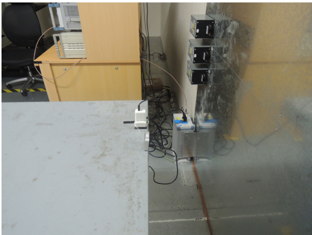
Photograph 7: Set-up for Mains Conducted testing (Back view)
