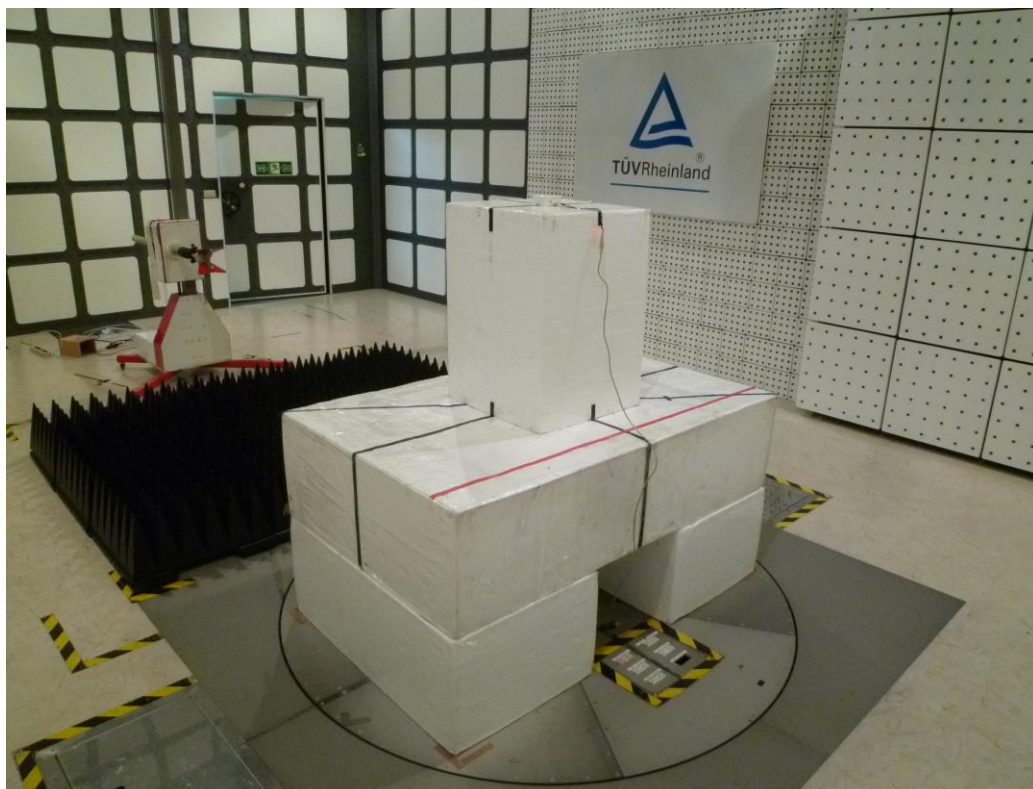
Photograph 3: Set-up for Spurious Emissions (Back View 2)
