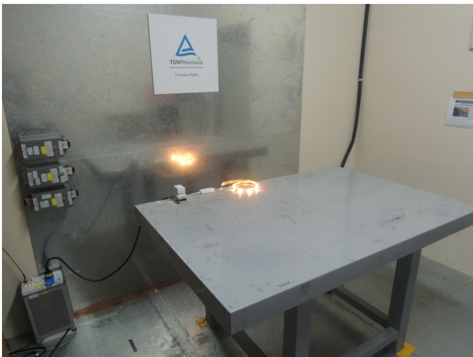
Photograph 8: Set-up for Mains Conducted testing (Front View)
