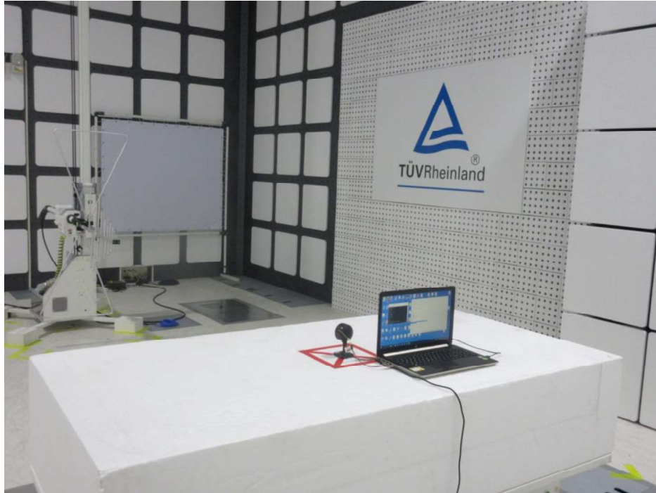
Photograph 5: Set-up for Spurious Emissions (Back View 3)
