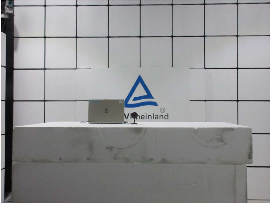
Photograph 1: Set-up for Spurious Emissions (Front View 1)
