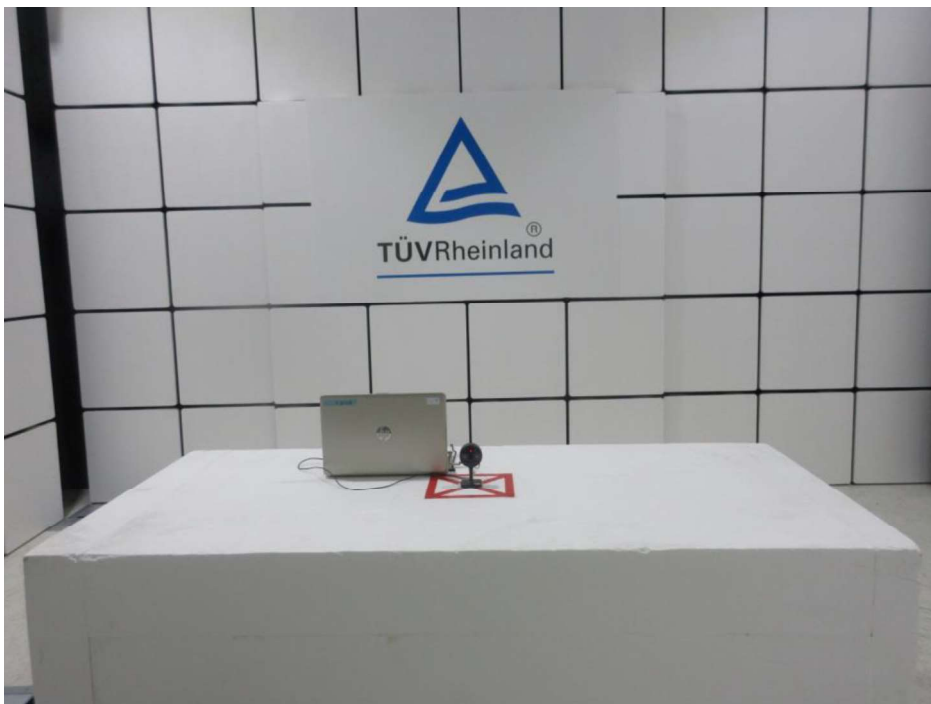
Photograph 2: Set-up for Spurious Emissions (Front View 2)
