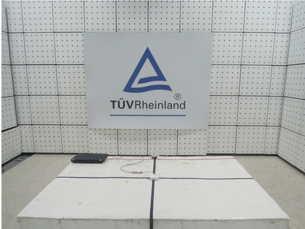
Photograph 2: Set-up for Spurious Emissions (Back View 1)
