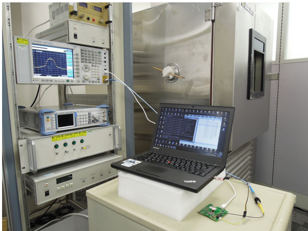
Photograph 4: Set-up for Conducted testing
