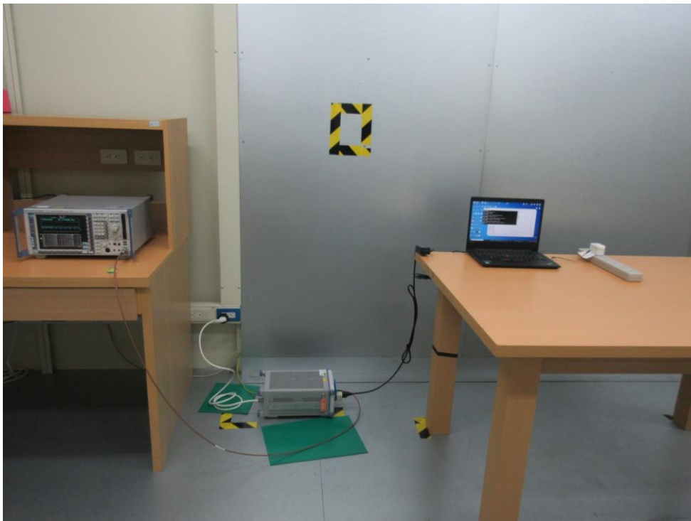
Photograph 7: Set-up for AC Mains (Front View)
