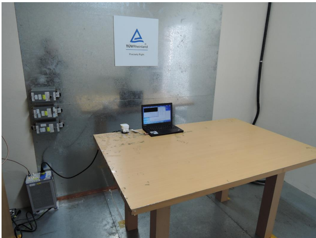
Photograph 7: Set-up for for Mains Conducted testing Front
