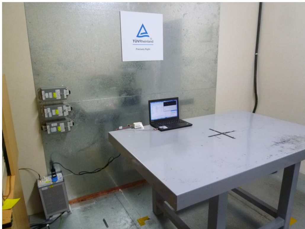
Photograph 7: Set-up for for Mains Conducted testing Front
