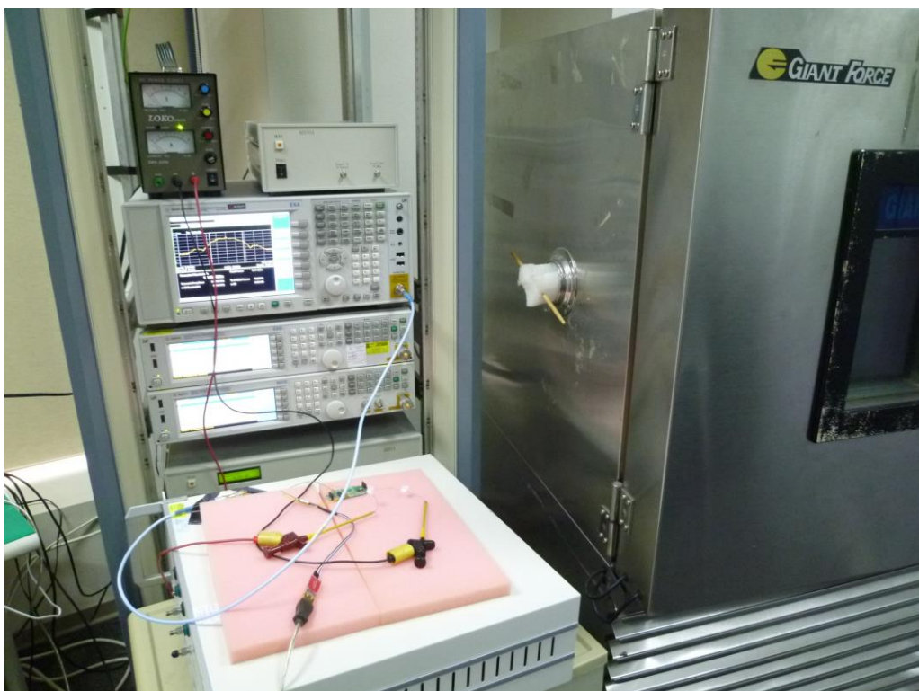
Photograph 5: Set-up for Conducted testing
