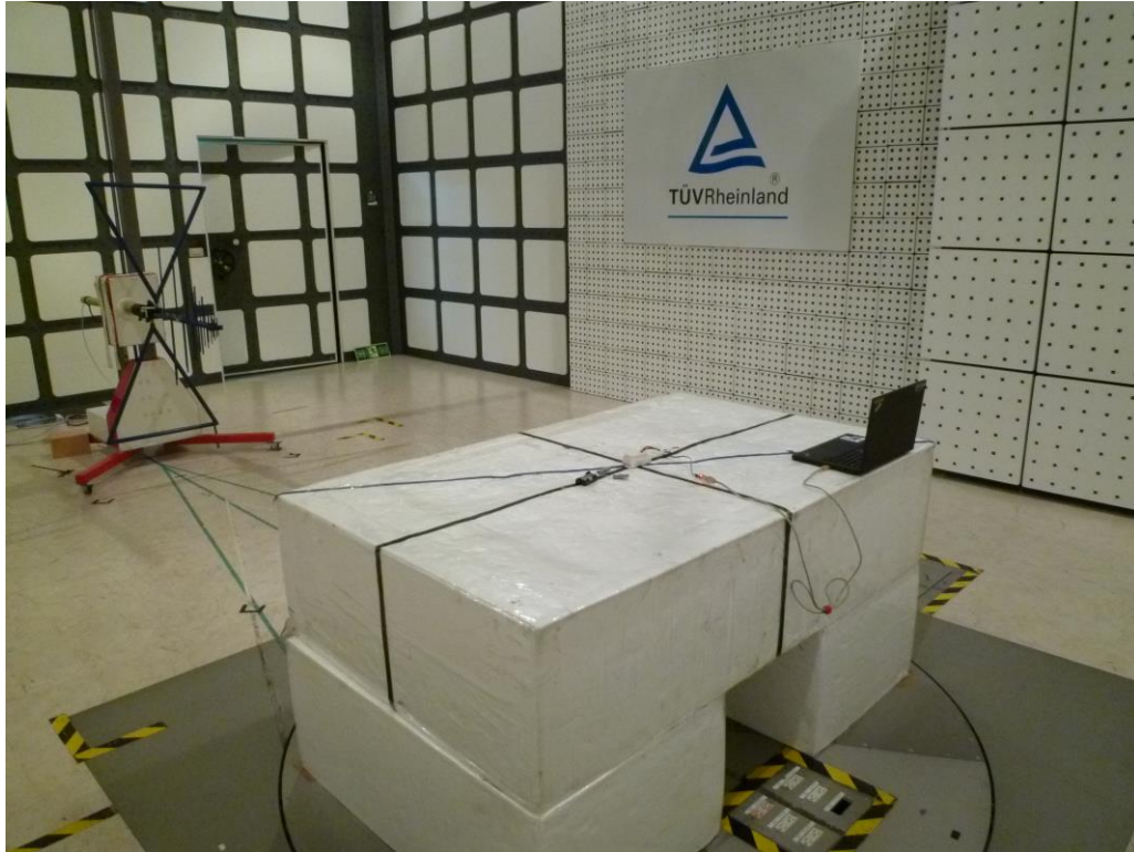
Photograph 3: Set-up for Spurious Emissions (Back View 2)
