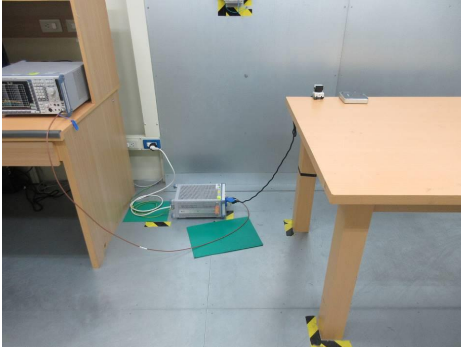
Photograph 7: Test Setup for Mains Conducted Emissions (Front View)
