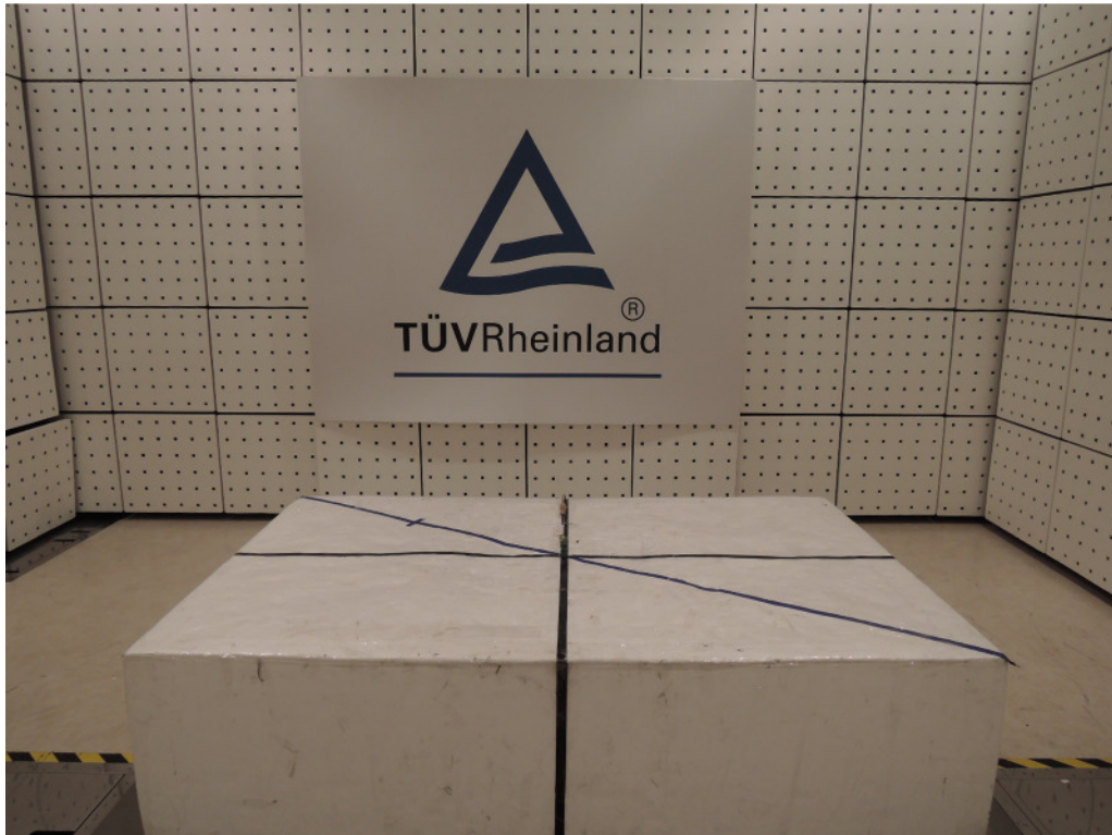
Photograph 1: Set-up for Spurious Emissions (Front View)
