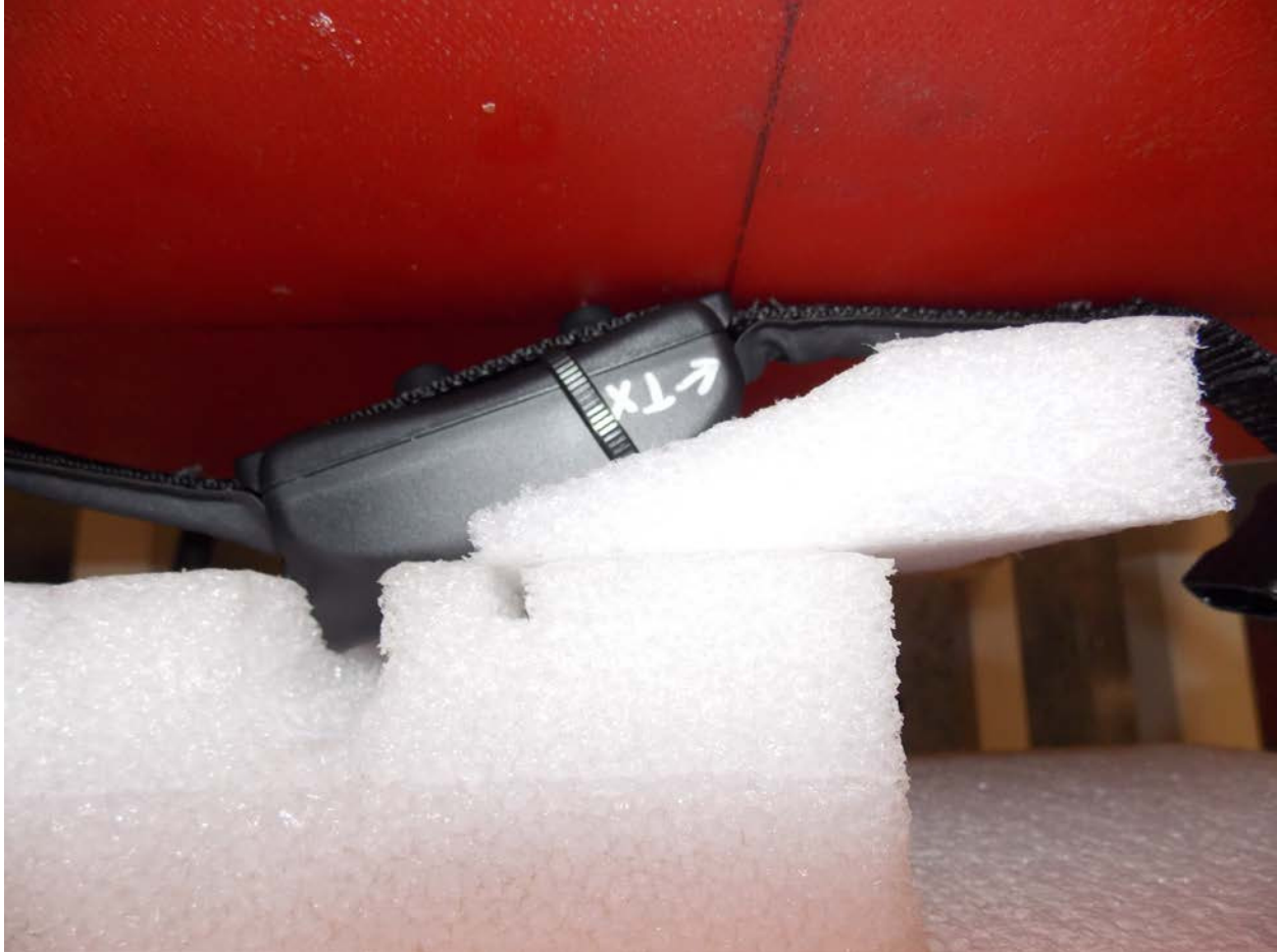
Test Position Main Antenna 0 mm Gap
