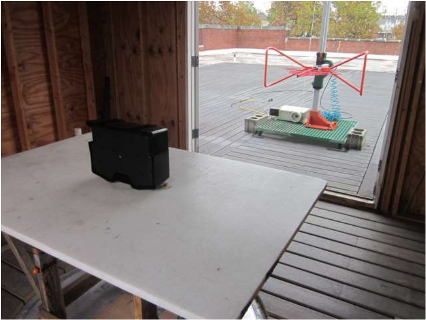
RADIATED EMISSIONS TEST SETUP 30-1000 MHZ 3 METER OATS
