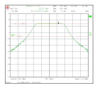
The peak level of 14.0 dBm is the maximum peak output of the Woodstream Model V430B Rodent Snap Trap with LoRa Radio. The conducted spurious emissions from the antenna port must be 20 dB down from this peak. The resultant limit is therefore -6.0 dBm and is displayed on the plots below.
