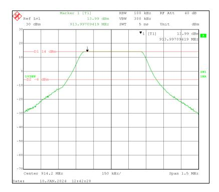
The peak level of 14.0 dBm is the maximum peak output of the Woodstream Model V430B Rodent Snap Trap with LoRa Radio. The conducted spurious emissions from the antenna port must be 20 dB down from this peak. The resultant limit is therefore -6.0 dBm and is displayed on the plots below.
