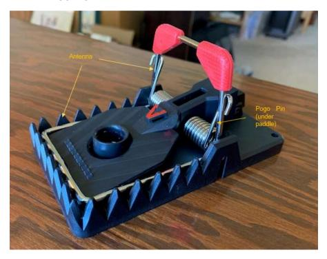
The antenna is the chrome plated steel wire bail that catches the rodent. A spring-loaded contact (pogo pin) on the PCBA conducts output to the pivot pin which conducts to the bail.
