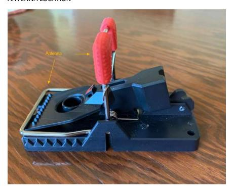
The antenna is the chrome plated steel wire bail that catches the rodent. A spring-loaded contact (pogo pin) on the PCBA conducts output to the pivot pin which conducts to the bail.
