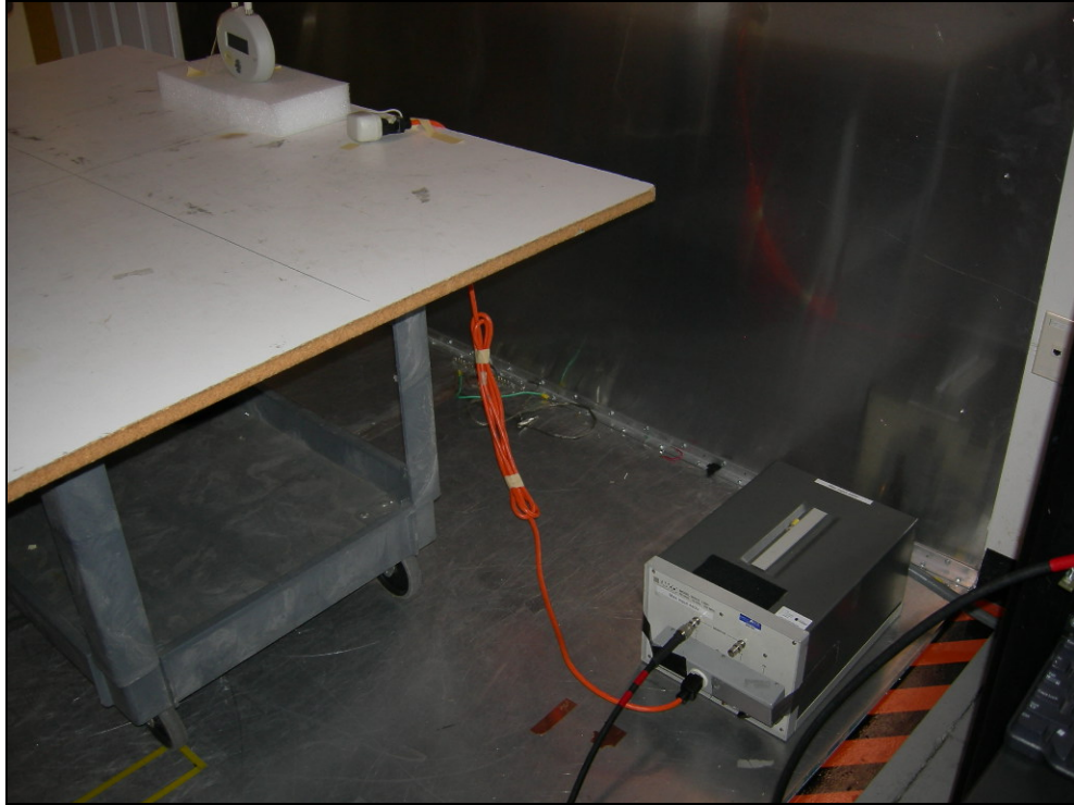
Figure 4: AC Power Line Conducted Emissions
