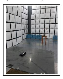
Radiated Spurious Emissions, 30 MHz to 1000 MHz
