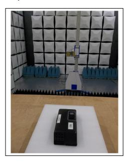
Radiated Spurious Emissions 18 GHz to 26 GHz
