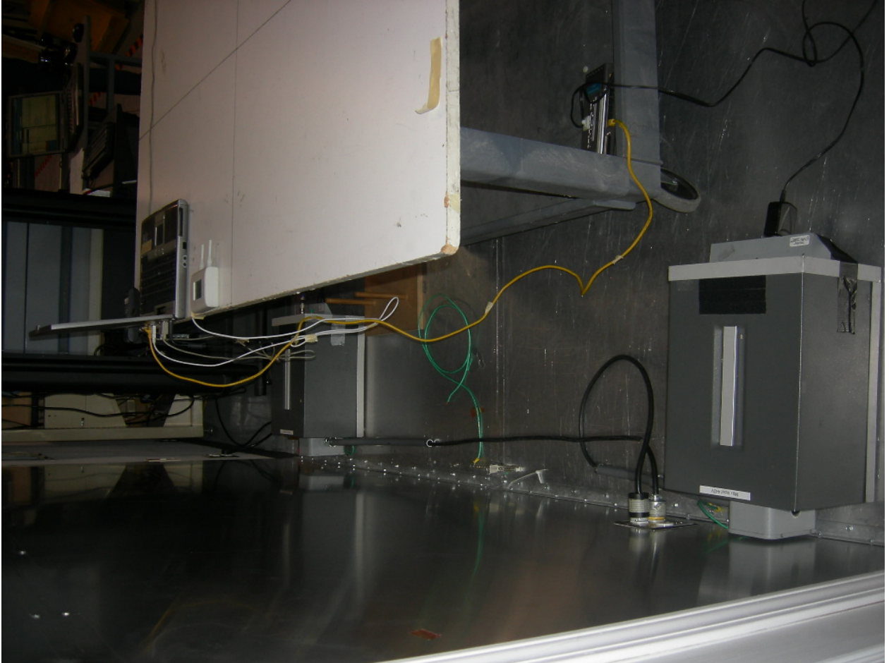
Figure 7: AC Power Line Conducted Emissions
