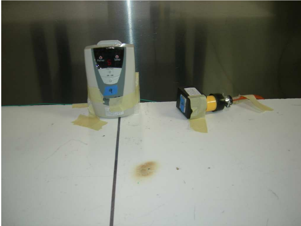
Figure 3: Conducted Emissions – Front View
