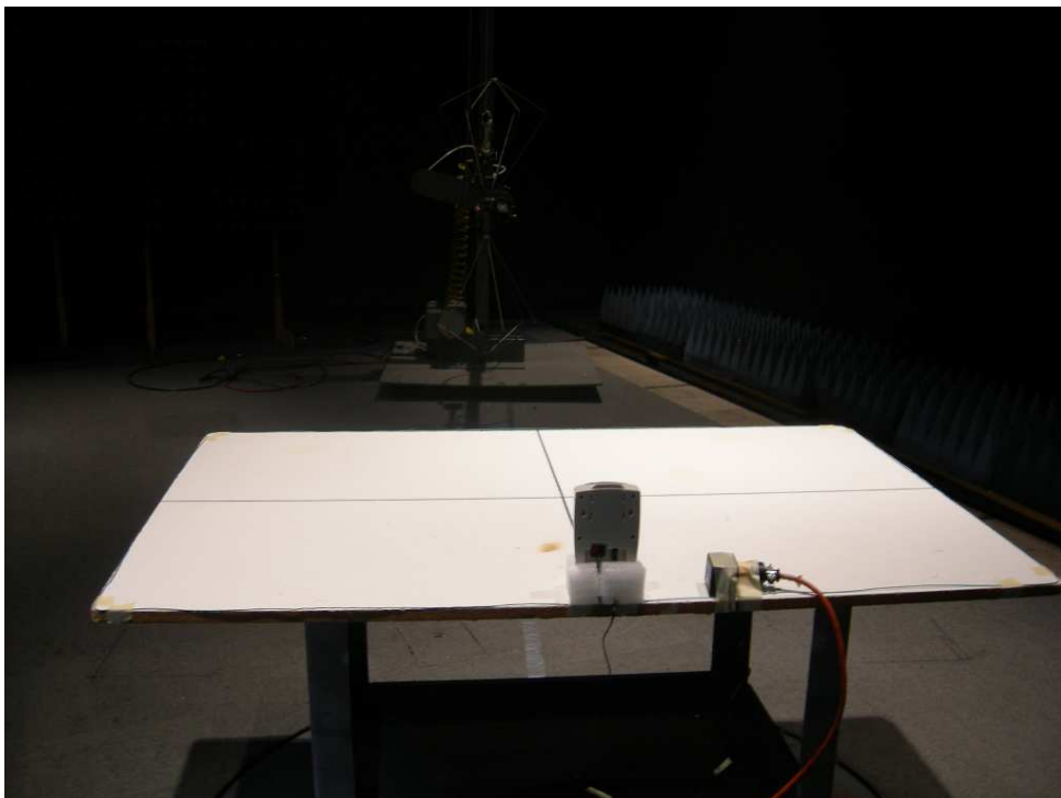
Figure 2: Radiated Emissions – Rear View
