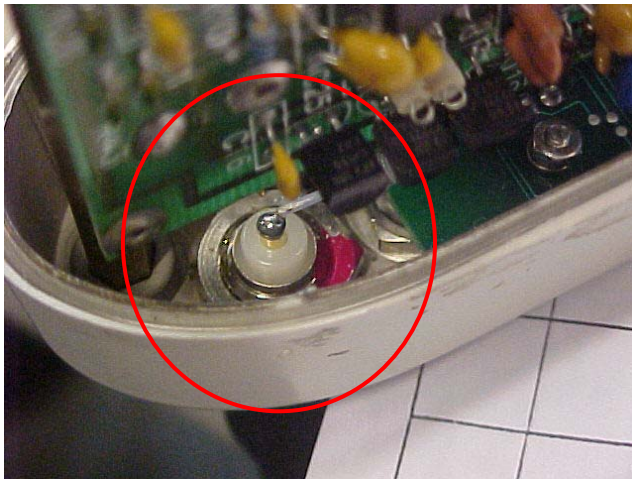
INTERNAL ANTENNA CONNECTION
